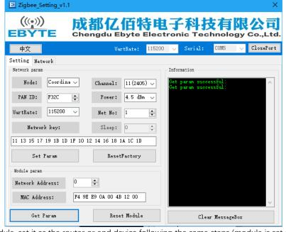
⑤.Select another module, set it as the router or end device following the same steps (module is set as end device when leave factory (default),no need to set again, in this experiment it is end device).
