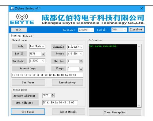
④.Select node type as coordinator, write in parameter. Wait the coordinator to start constructing network and users can check module parameter.
